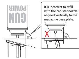
Please turn the magazine up side down to keep the injection hole side up, fill the gas only when the canister is verticalized to the injection hole. The gas will not be filled into the magazine or will leak out if the canister is not verticalized to the injection hole.
