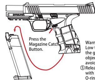
Warning - Attention! Low temperature gas will be vented out while releasing the gas. Never point the Magazine Nozzle Seal towards any object that you do not want to damage while operate to avoid frostbite. Release the remaining gas by pressing the Magazine Valve with either finger or tool, to avoid elastic fatigue of your O-ring.
