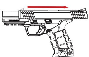
② Push the Slide to the end of the rail, then release it for repositioning.
