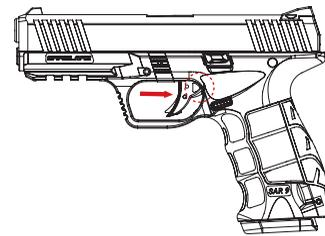
The Trigger Safety needs to be pressed properly to fire normally.
